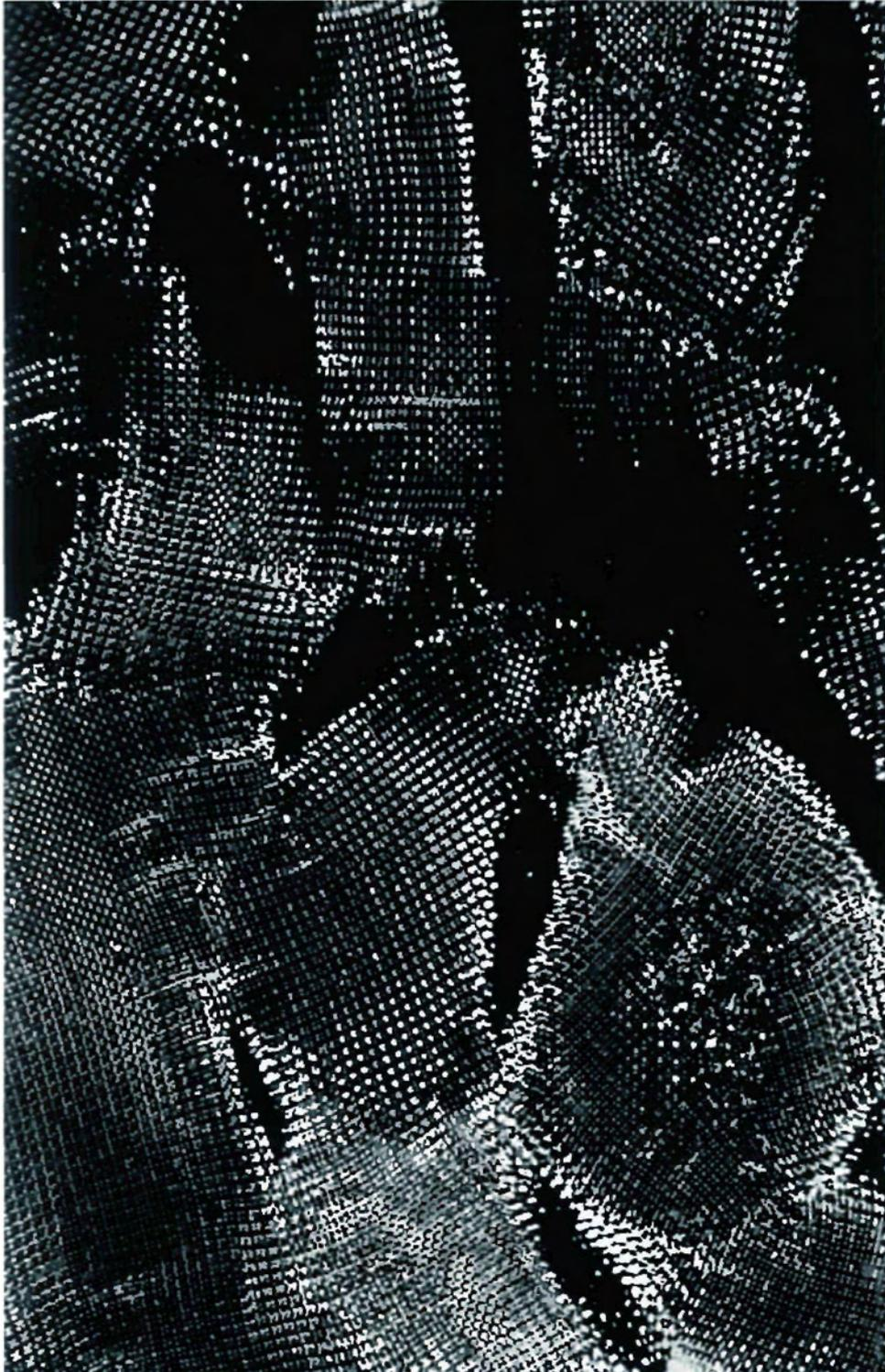
53 When the pattern produced by vibration is as delicate as this, it may be appropriately termed a texture. These wave fields are produced in a layer of glycerin on a diaphragm excited at a frequency of 300 cps. Here again many parts must be imagined in motion. Labile waves appear, particularly in the marginal areas of the textures, and often look like turbulences.
