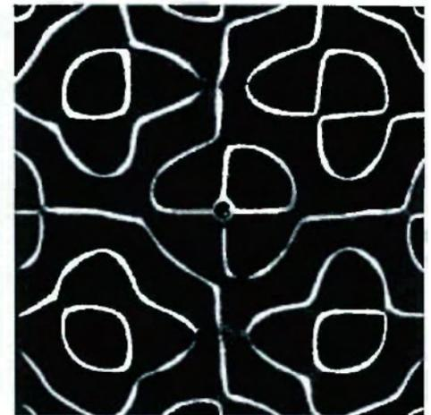
1-6 The illustrations show a simple sonorous figure taking shape under the action of crystal oscillators (piezoelectric effect). Steel plate 31x31 cm. Thickness 0.5 mm. Frequency 7560 cps. The material strewn on the plate is sand which has been calcined to purify it.
