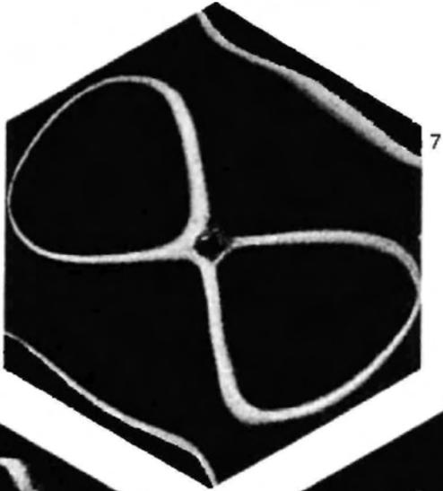
7-11 In figures 7 and 11 a single tone (800 cps in Fig. 7, 865 cps in Fig. 11) has produced its own sonorous figure on a hexagonal steel plate. Figure 9 shows the result when both tones are sounded at the same time and at equal strength. Figures 6 and 10 show the intermediate stages.
