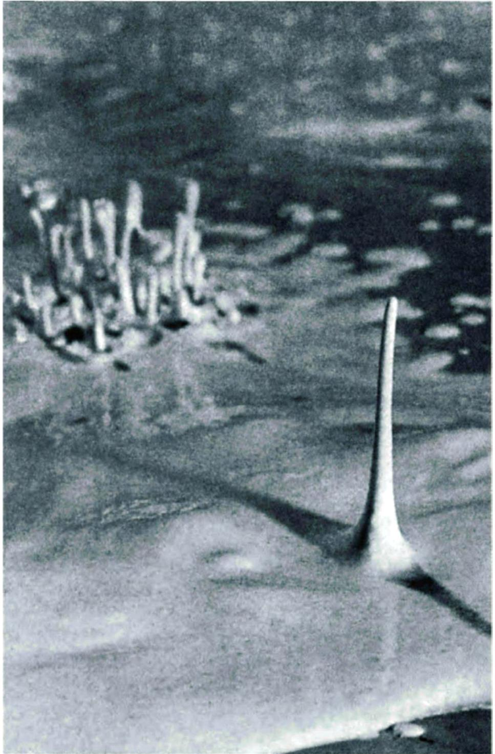
142 In experiments with "solidescence," curious effects resulting in figurines are repeatedly observed. The tall, columnar figure is driven up by vibration. At the time the photograph was taken, the mass was still viscous. Although the figure persists for some time it will vanish in the course of the experiment as the material enters the solid state. Other morphological elements will also appear as the result of vibration.
