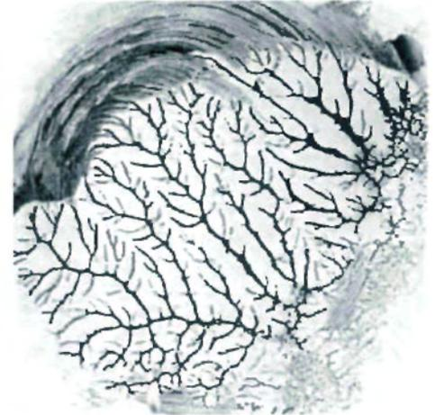
99, 100 If a doughy mass is pulled apart, the surfaces do not reveal a random but rather a characteristically organized pattern. This phenomenon of dehiscence produces tree and branch-like patterns, delicate filigrees and fine networks. The branch work in figure 99 is sometimes thick, but in figure 100 (he dendritic pattern is more delicate.
