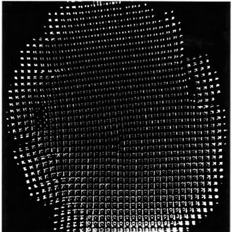
50 "Standing" lattices showing great regularity in their features may appear in oscillating sheets of liquid. Glycerin has been poured onto the diaphragm as a liquid layer.
