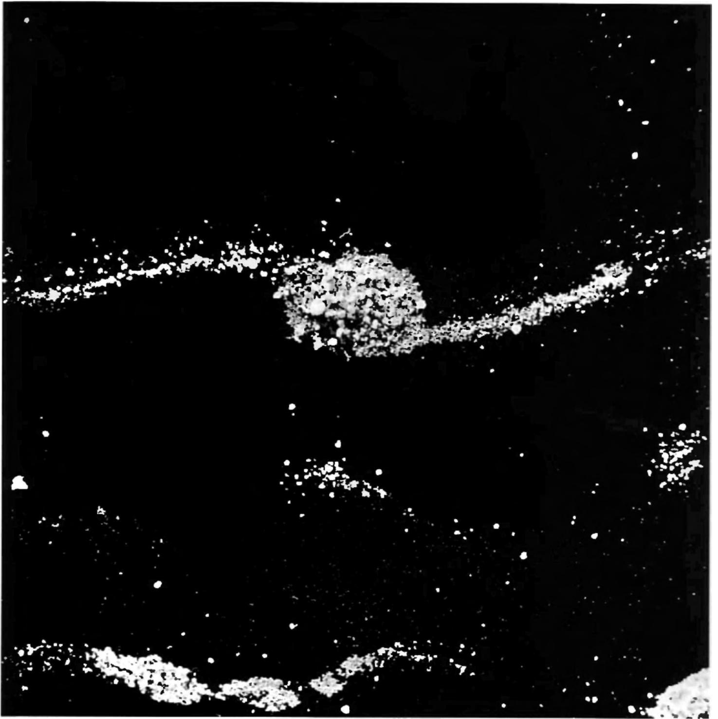
27-30 The four figures reveal approximately the same pattern but the number of elements grows as the pitch increases. In figures 27 to 30 the frequencies are 1690, 2500, 4820, 7800 cps, respectively. Steel plate 23x23 cm. Thickness 1mm.
