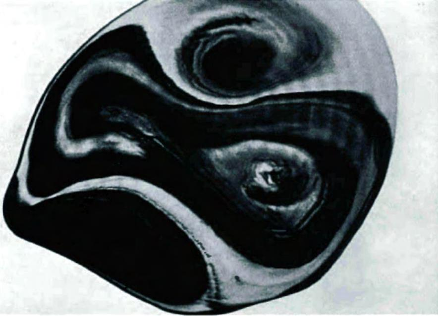
65 Hydrodynamic phenomena originating in vibration are a rewarding field for observation. In addition to vortices other new patterns can be found. In figure 65 a figure-eight form can be discerned; there is however no intersection as in a lemniscate. The effects of sound have produced circulation.
