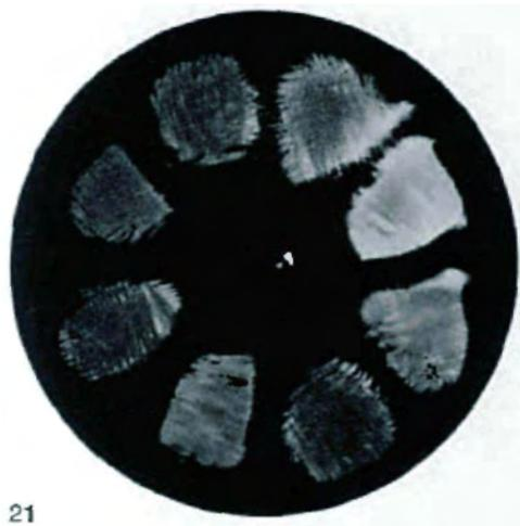
21 The same plate excited by the same frequency as in figure 20 but covered with a liquid. Now the areas of movement (antinodes) are visualized directly as wave fields.
